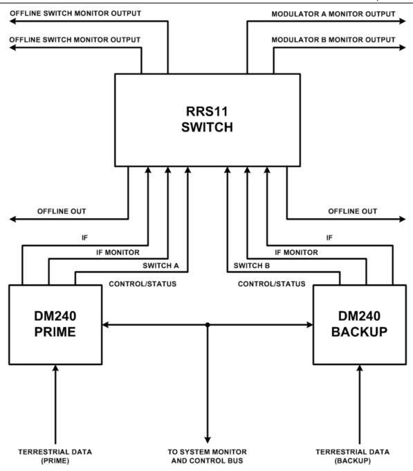
Figure 3-1 RRS11 Functional Block Diagram
